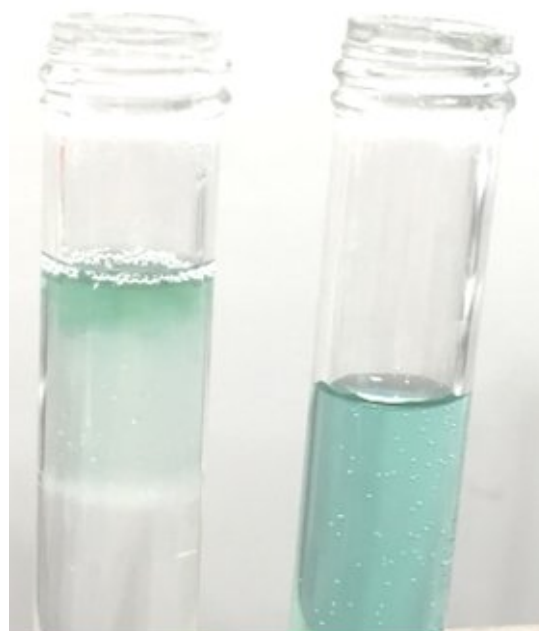
Fig. 1: Aqueous solution of sunset yellow FCF and brilliant blue FCF. Before extraction process (right) and after CPE method (left). Two dyes are transferred to surfactant-rich phase.
